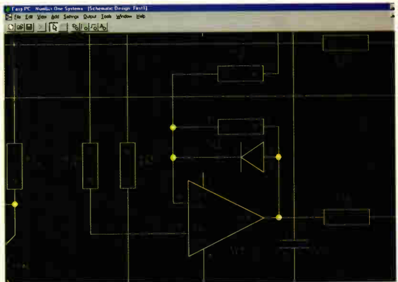
Fig. 1. Close-up view of a schematic drawing, showing the new Windows controls. Note the balance between icons and menus and how similar the symbol/drawing style is with previous versions.
