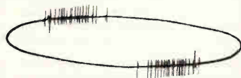
Fig. 9. Photograph of ERA Model 3 on-screen results. The test voltage considerably exceeded the capacitor's discharge inception voltage. Display shows multiple ionisation discharge pulses, surrounding a calibration pulse. Note discharge pulse amplitude is relatively unchanged by this change of applied voltage, but pulse count has increased.
