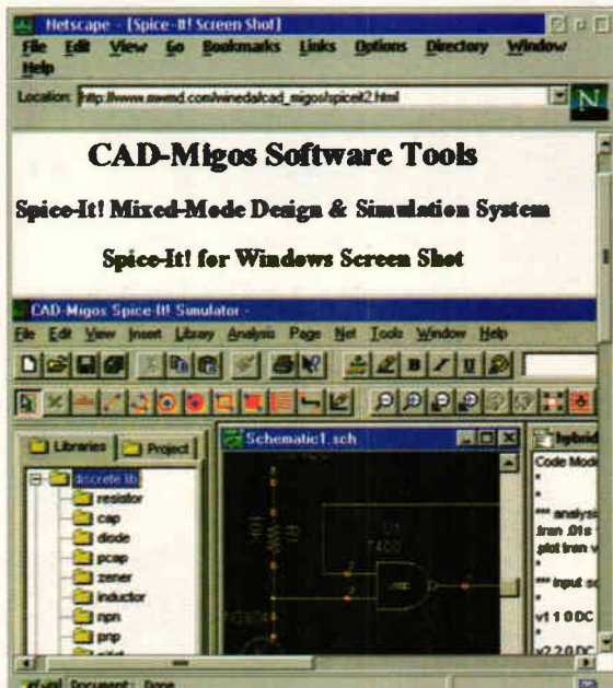
Fig. 6. The 'Spice-It' simulator is based on the XSpice core, not just Berkeley Spice. Yet it remains fully compatible with Spice 3F5 simulators.
