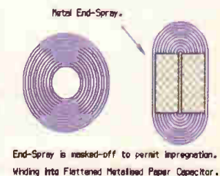
Fig. D. Stages in making a "flattened" capacitor. The original metallised paper element (left) is wound using a larger than normal spindle diameter, in order to facilitate flattening to the finished shape (right).
