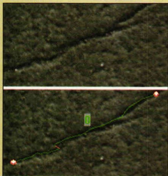
Shown (left) is the post processing crack detection algorithm. This takes into account a crack's typical line proportions, and involves interpolation between points. Also shown is a block diagram of the road inspection system. The camera input is mixed with road locational data before being scan converted for recording on video tape or for digital signal processing before being store on a pc's hard disk drive.
