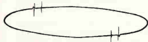
Fig. 8. Photograph of ERA Model 3 on-screen display. The test voltage slightly exceeds the capacitor's discharge inception voltage. Display shows a single ionisation discharge pulse, immediately preceded by the calibration pulse.
