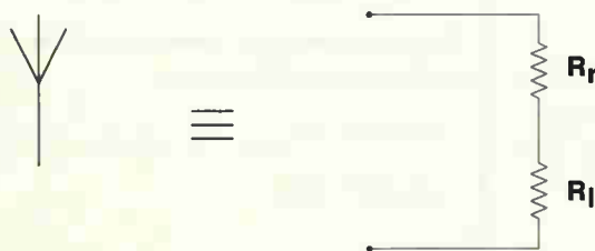
At resonance, a tuned antenna looks resistive.
