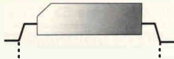
Fig. 3. Bending down the leads of a SOIC package gives you an extra 0.02in of clearance on either side of the pin.
