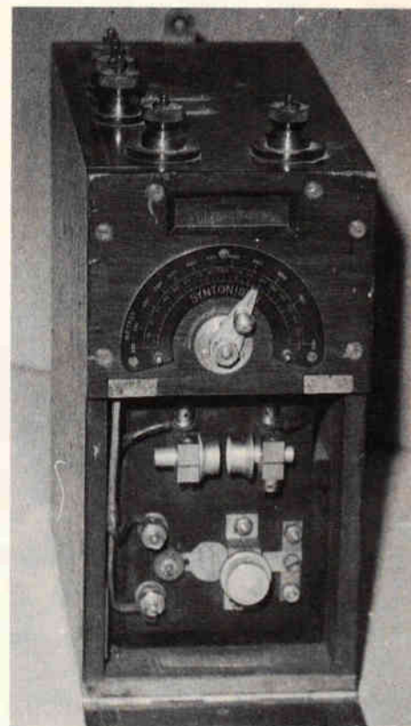
Photo 3. Transmitter for aeroplane wireless station from circa 1915 – one of the first transmitters designed specifically for aviation.
