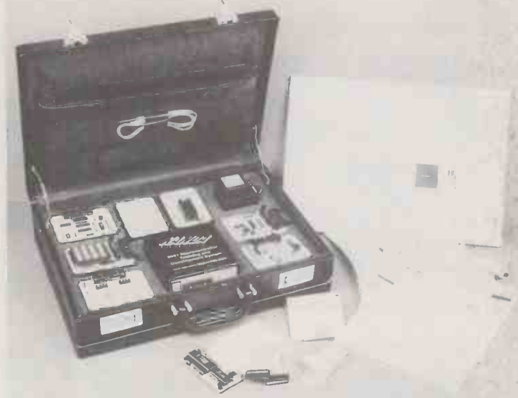
All elements of hardware and software of the microcontroller training kit are housed in the same lockable case.
