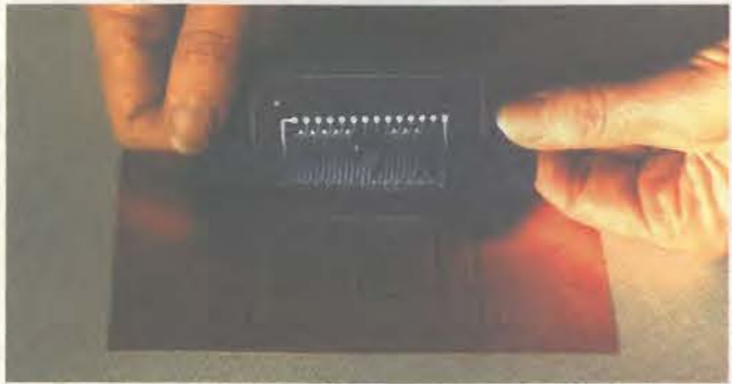
After being passed through a pouch laminator, the PnP sandwich is peeled off by hand.
