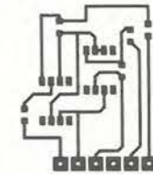
Fig. 2. Actual size of a surface-mount board showing that plotters are capable of fine detail.
