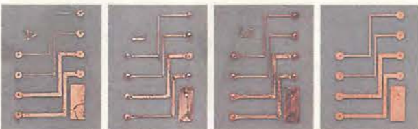
Results of plots made with various inks intended for overhead projector work are shown in a), b) and c). Very poor etch resistance is indicated. Plot d) was produced using proper etch-resistant ink. Not shown is a further plot produced using waterproof Indian ink: the copper was completely etched away.
