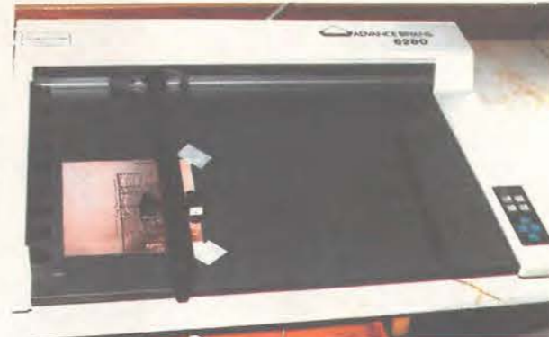
Plotting with a 0.3mm pen directly on to 0.35mm copper board. Note that the board is clamped on the left-hand side and held flat on the right using masking tape – not the usual magnetic strip.
