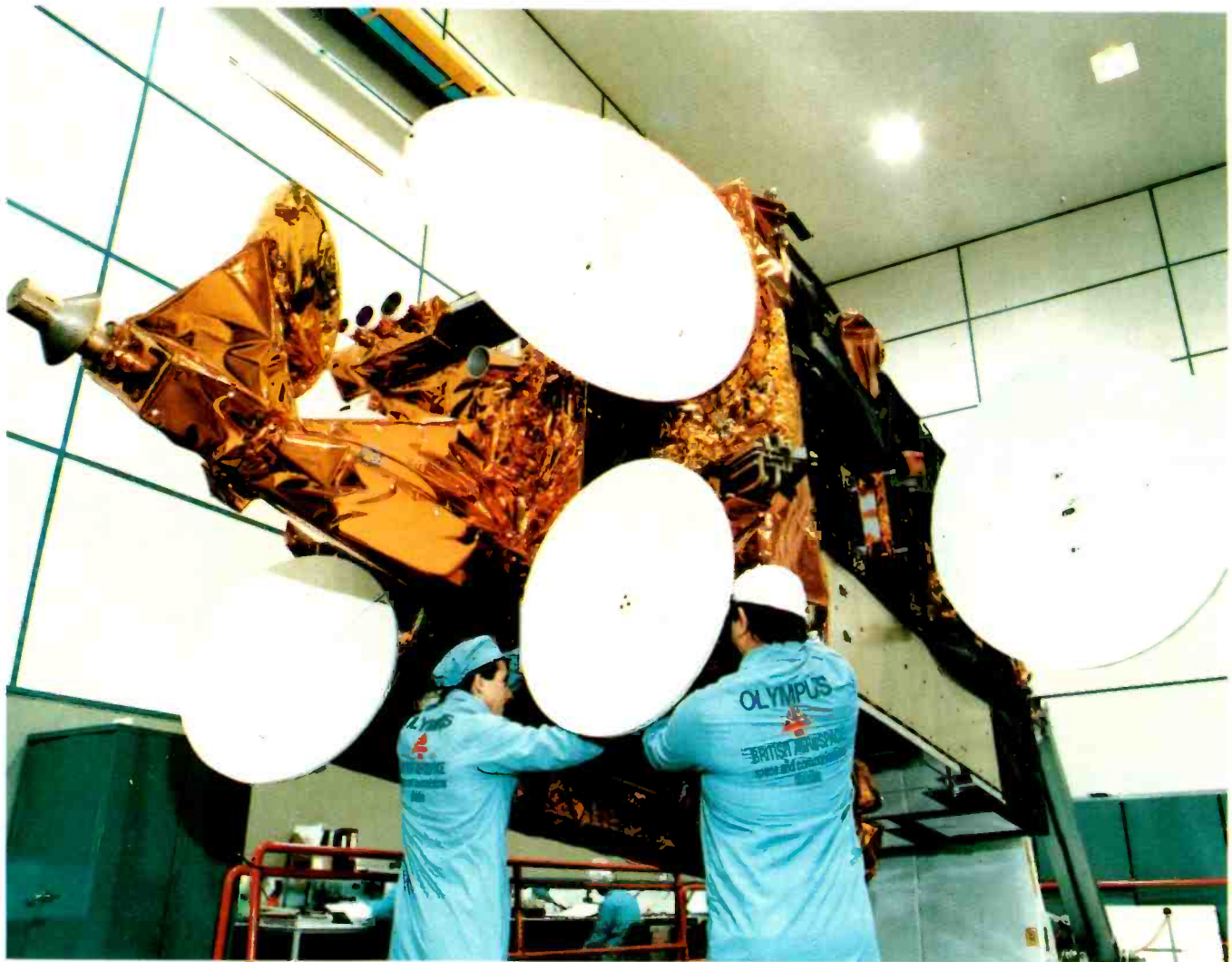
Olympus is to be used mainly for television broadcasting. Weight at launch was 2617kg, the power available at the beginning of life 3600W, and the solar arrays 26m end-to-end. This satellite is claimed to be the largest civil communications satellite ever launched. Photo ESA.
