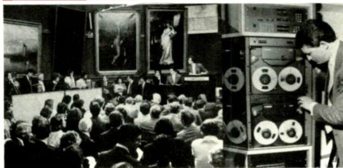
All bids made at a Christie's London auction are recorded on tape by this 22-channel voice logging system from Philips which records the incoming bids from 17 telephone channels as well as the auction room bids and the auctioneer's voice.
