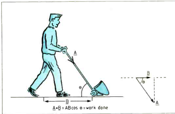
Fig.6. Work done by the component of a force shows a typical example of the scalar product of two vectors.
