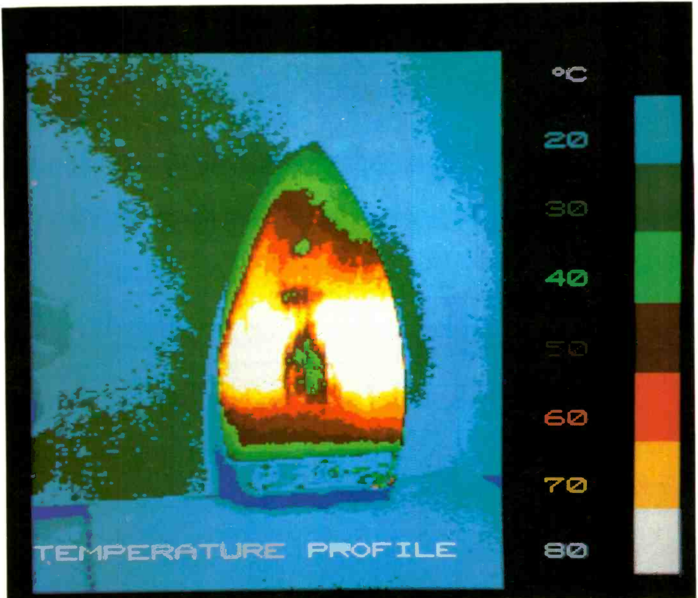
With the colour palette, monochrome images can be coloured in up to 16 shades from a range of 4096.
