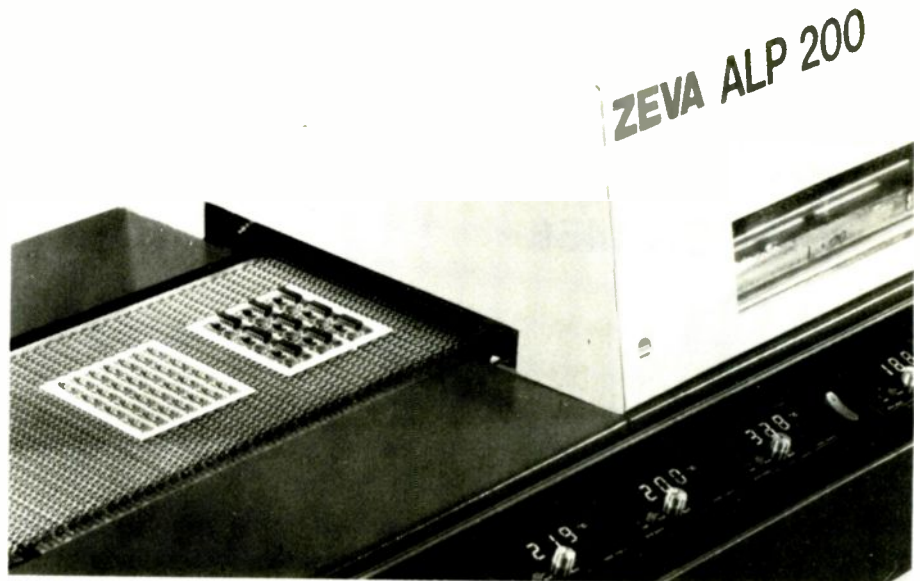
A reflow and curing oven for surface-mounted devices. Four heating zones can vary the heating cycle profile. — Zevatron GB, Dover.
