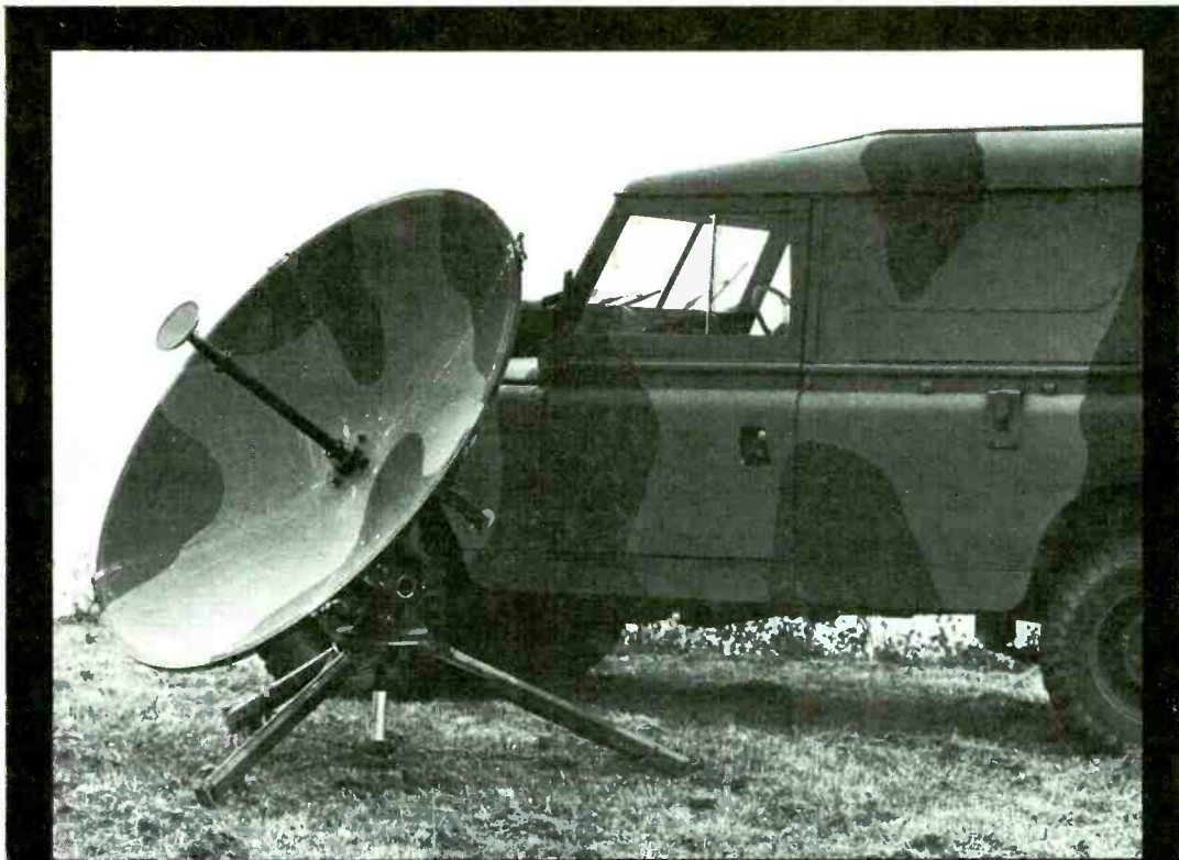
A prototype of what is said to be the first mobile satellite communications ground station from Racal-SES. The company are to supply the MoD with a number of such stations for use in military communications from a forward headquarter position.
