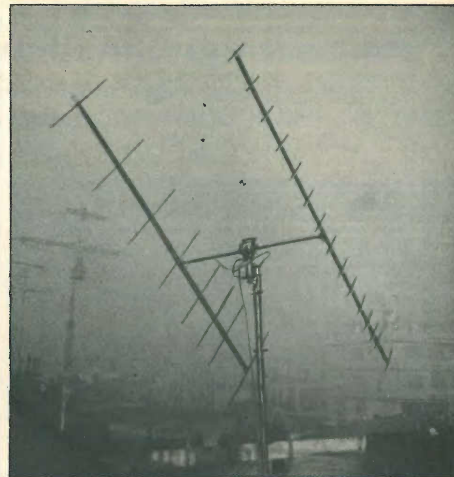
This aerial system is used by the author for tracking Oscar satellites. The aerial to the left is for 145.9MHz and the one to the right for 435.1MHz. Both aeriels are mounted on the same shaft supported in the middle by the elevation rotator which is mounted on the azimuth rotator.
