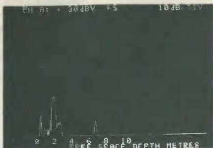
By taking a radar picture of the ground and then subtracting that from the composite picture of the ground with pipes, it is possible to leave a picture of the pipes.
