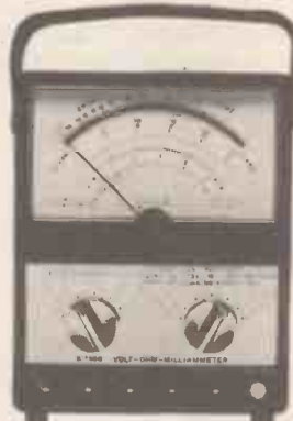
K 1400 Multimeter 20,000 OPV. DC and AC volts up to 5000. DC and AC amps up to 10. Resistance up to 20 megohms. "Off" damping. Overload protection. R.R.P. £79.35 ex. VAT.
