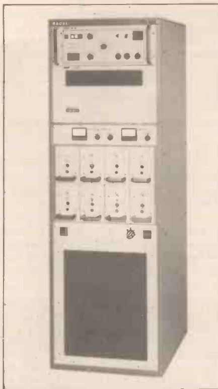
Fig. 2. Solid state 1kW transmitter comprising eight 125W modules.
