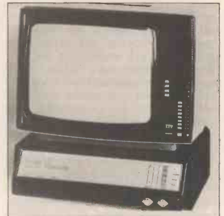
ITT TXV 16 viewdata terminal. The lower section contains an isolated power supply and the viewdata equipment while the upper section can function as either the viewdata display or as a "straight" 16in black and white tv receiver. ▼
