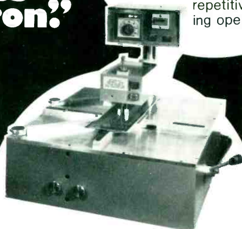
Multicore Solderability Testers. MK III - Tests components semi-automatically. New PTH - tests plated-through-holes in P.C. boards automatically.
