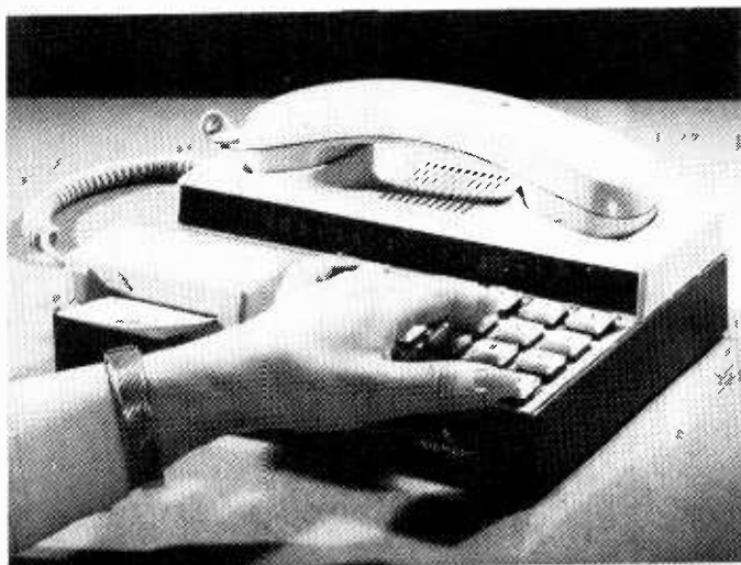
This push-button data telephone with visual display has been developed by Siemens, Munich, as a result of a study of the 'human factor'.
