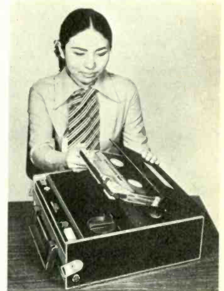
The Panasonic (Matsushita) magazine loading v.t.r. The unit is built to the specifications laid down in the Japanese Type I Standard for \frac{1}{2} -inch video tape recorders. The magazine illustrated contains enough tape for recording and reproducing a 30-minute programme.
