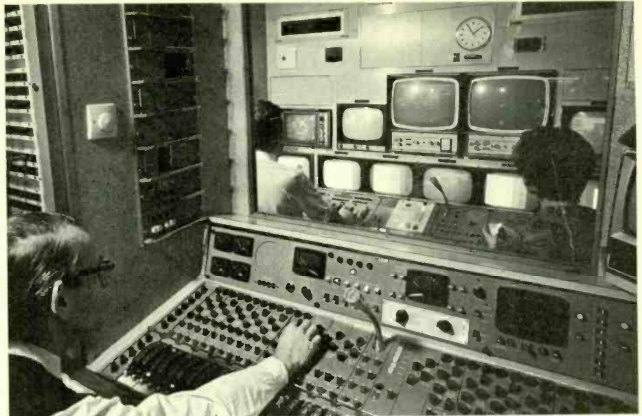
Granada Television Network officially took possession of the first of its fleet of colour television outside broadcast vehicles on 2nd December. This is a 5-camera mobile unit which has been designed and built by EMI to meet the special programme requirements of Granada. The picture shows the view from the sound control position into the production control area.
