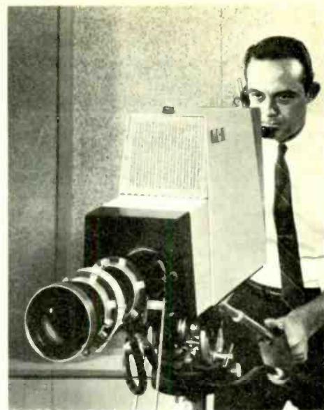
The single-tube colour television camera from R.C.A.
