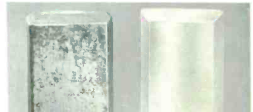
A section of a typical cast solder bar. Note the surface dross and general contamination.
