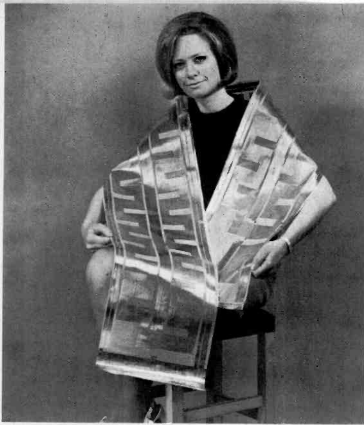
Not a new line in stoles, but illustrating the general appearance of a length of printed conductors before winding.
