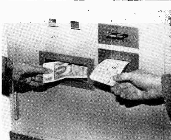
Cash after the bank has closed will soon be a possibility on the continent due to an automatic paying out machine developed by Telefunken in co-operation with Ostertag-Werke AG. The bank issues the customer with an identification token for use with the machine as well as a punched card. The equipment compares the punched card with the identification token and then pays out a 100 mark note.
