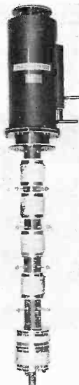
This English Electric u.h.f. klystron will operate at the high peak output power of 40 kW.
