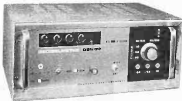
Numerical indication of signal level in decibels with respect to 0dB reference (1mV into 600 \Omega ) is given by this Compagnie des Compteurs instrument designed for the range 10 c/s to 100 kc/s.
