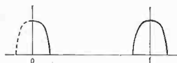
Fig. 3. The low-pass function is translated in n -path filters to a band-pass function centred about frequency f .
