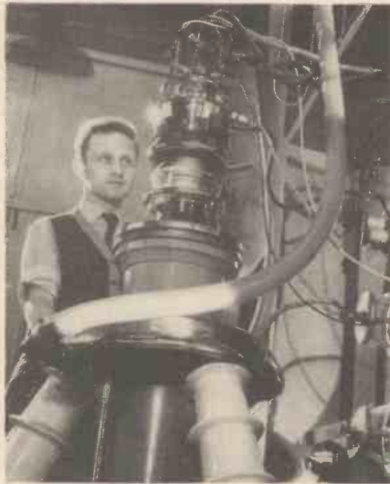
After being high-voltage tested at Standard Telephones and Cables factory at Paignton, Devon, this 150 kW triode valve is to be exported to Sweden. It will be used in a high-power broadcasting transmitter.
