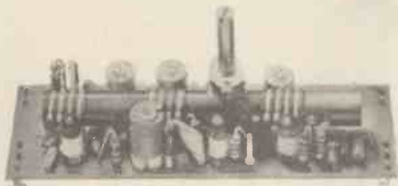
Silicon planar transistors in a three-gang inductively tuned circuit are used in the v.h.f. input circuits of the Graetz "Silvretta" stereo receiver.
