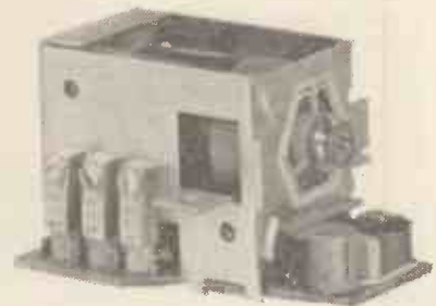
Below.—"Brushless" d.c. motor and switching transistor panel as used in the Grundig cassette tape recorder
