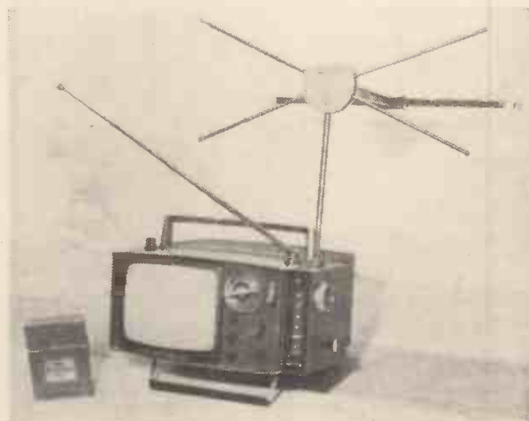
Sony transistor portable showing telescopic v.h.f. aerial and u.h.f. adaptor (right) with its plug-in foldable aerial.
