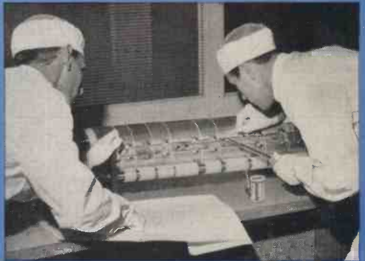
Ersin Multicore Solder is shown being used at the Erith factory of Submarine Cables Ltd., in the production of a submersible repeater designed to last for a minimum of 20 years under the sea without attention.
