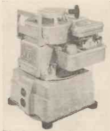
This portable petrol-driven electric power generator shown by McCulloch Mite-E-Lite Inc. uses a rotating permanent magnet to overcome brush problems and increase efficiency. Weighing 55 lb, it produces 650 watts.
