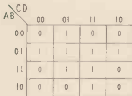
Fig. 17. Karnaugh map with a number of possibilities for looping two terms.
