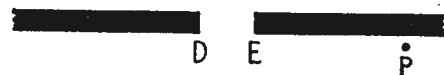
Fig. 4. Although opposite sides, D and E, of this wider opening are in phase as regards the original source of waves, their wavelets reach P out of phase, tending to cancel one another and reduce diffraction.
