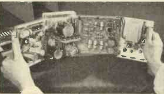
Marconi Instruments a.f. oscillator opened for servicing. Instrument still works in this form.
