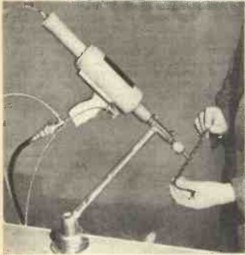
Riveting machine by Chobert (marketed by Avdel), for quick insertion of rivets and solder tags into metal and plastic. Tool is pneumatically operated.
