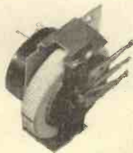
Airmax axial-flow blower, claimed to be the world's smallest, moving about 5cu ft/min at 1,000 r.p.m. Power supply is 26V, 400c/s, 3-phase.
