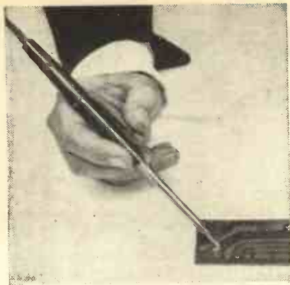
Enthoven "Miniscope" soldering iron using a 2.5 to 6V supply. The heating time is five seconds, the iron is switched on by depressing the lever.
