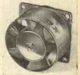
Airmax axial-flow blower, claimed to be the world's smallest, moving about 5cu ft/min at 1,000 r.p.m. Power supply is 26V, 400c/s, 3-phase.
