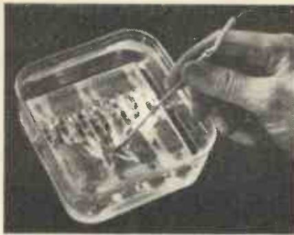
Left: Circuitry encapsulated in Midland Silicones gel Type DP2603
