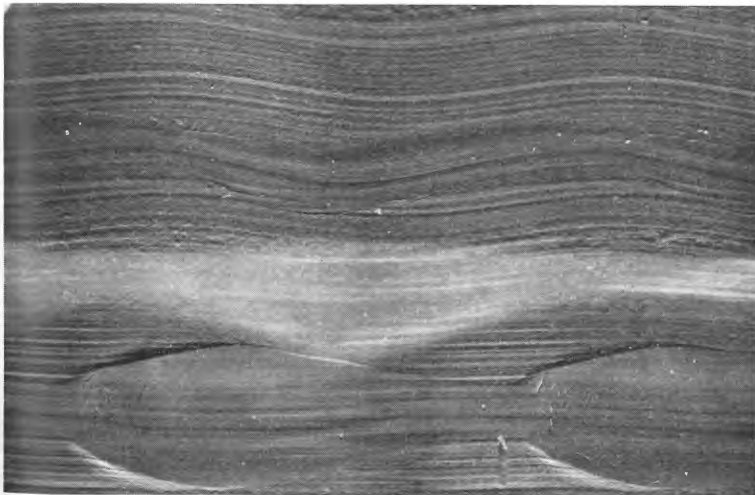
Fig. 3. Same groove as Fig. 2(a) after 5 consecutive playings with same stylus shows very little further deformation. The stylus track on the unmodulated wall is however clearer.
