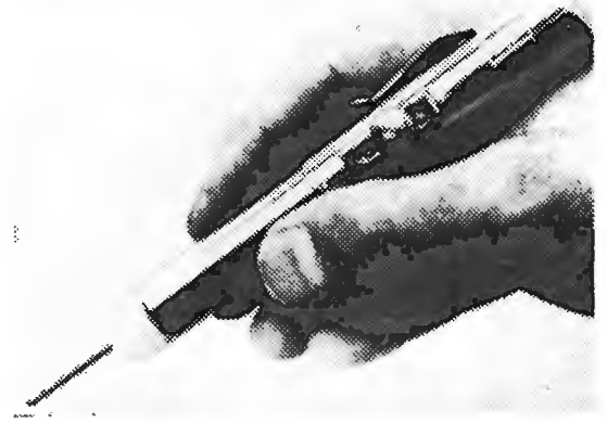
Pensource pocket test oscillator. On-off switch is near the pocket clip.
