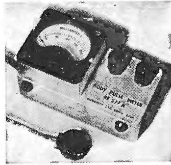
Pulse rate meter by Burndeft, showing carbon transducer.
