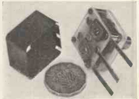
Right: Jackson Brothers Type S.D.1 miniature tuning capacitor.
