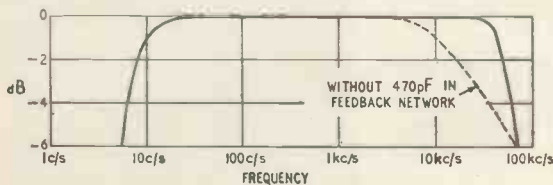
Fig. 3. Small-signal overall frequency response of 4-W amplifier.
