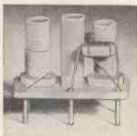
Plessey first i.f. 10.7 Mc/s f.m. transformer in which the coupling can be varied (by moving the core in the centre former) without altering the tuning of the two outer cores.
