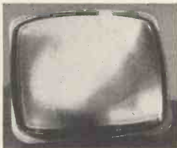
Integral-safety-shield television c.r.t. by Cathode Ray Tubes Ltd. "Ears" at corners ease mounting problems.
