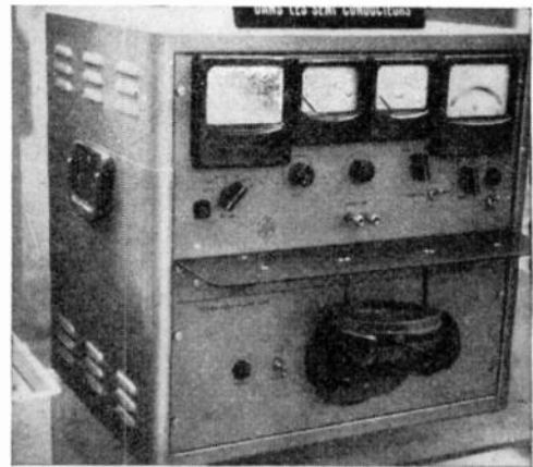
Test instrument for routine measurement of carrier lifetime in semiconductors (J. L. Amiot).
