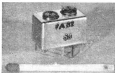
Below: Pair of i.f. coupling transformers for transistor printed circuits. Q > 160 ; dimensions 20 x 13 x 13mm (Orega).
