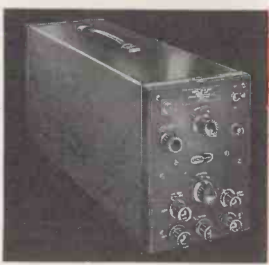
MODEL 1447 For delaying the work voltage to standard oscilloscopes until time-base has fired DC to 11Mc/s—0.5μsec delay DC to 8 Mc/s—1μsec delay
