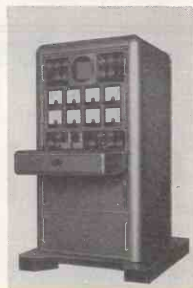
MODEL 1442 Laboratory high-gain amplifier for use in industry, nuclear physics, neuro and myo-graphic investigations response: 5c/s to 3kc/s gain: 10 4
