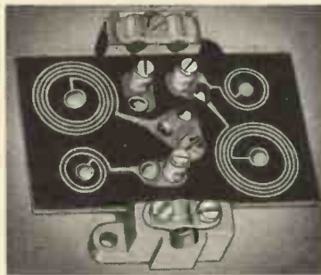
The interior of an L.1360 TV/FM diplexer is shown in this photograph. The continuity of the outer braid is maintained through the metal body to which the board is secured.
