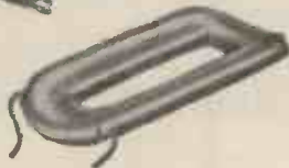
3 Field Coil for motor car dynamo wound with 280 turns of .030 inch enamelled wire.
