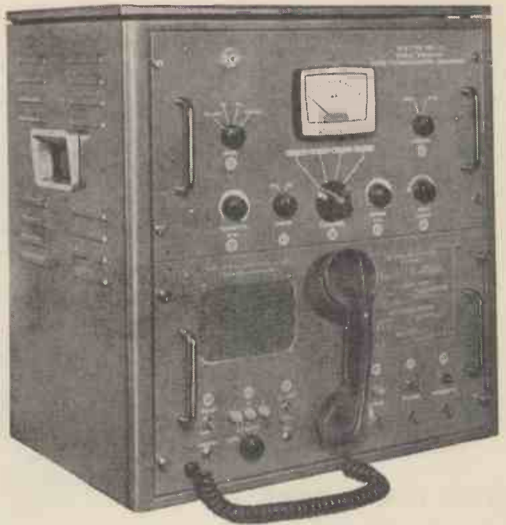
SSB-L1 Fixed Station. 60 watt (500 watt double sideband equivalent) eight channels 3-15 mc/s.
