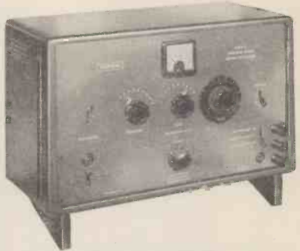
MUIRHEAD D-695-A OSCILLATOR Frequency Range : 10 c/s — 31 Kc/s
