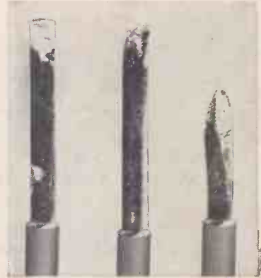
▲ The left hand bit was used with Savbit alloy and has made 10,000 joints. The centre bit was used for 1,000 joints and the bit on the right for 7,500 joints, each with a standard tin/lead alloy.
