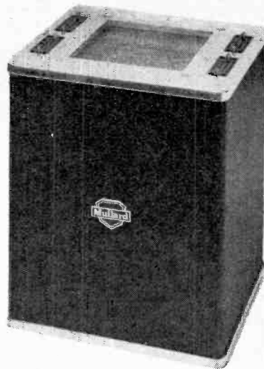
Magnetic-core matrix store (Mullard) used in many computers for immediate-access storage. The box contains a stack of matrix planes.
