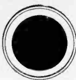
Fig. 5. In the circuit formed by a wire ring around a core carrying a varying magnetic flux, a current flows without any difference of potential or accumulation of charge.
