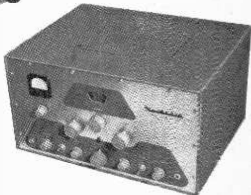
DX100 (Heathkit) 15-valve 100-W transmitter for amateur bands. The Modulator uses a pair of KT88s in the a.f. output stage.
