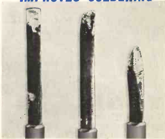
Under controlled conditions the bit on left, used with Savbit Alloy, made 10,000 joints. Centre bit, used for 1,000 joints and bit on right for 7,500 joints, were used with standard tin/lead alloy.
