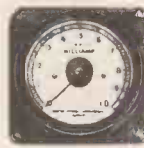
"Fulscale" meter 4 in. dia. scale moving coil having 270° arc with a 9 in. scale length.
