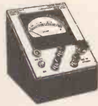
Ohmmeter for the rapid and direct measurement of very low values of resistance. Model RM.155.
