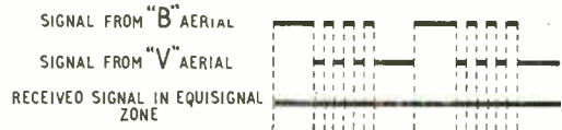
Fig. 2. The equi-signal course path arises from the overlapping of the B and V morse signals radiated by the two aerials.
