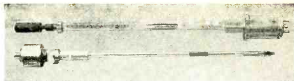
English Electric travelling-wave tubes N1001 and N1002
