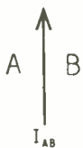
Fig. 3. The convention adopted herein is that I AB is positive when flowing in the direction shown.
