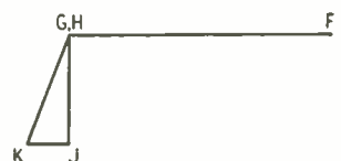
Fig. 5. Completed voltage and current diagrams for Fig 2 at balance.
