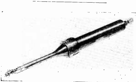
This new electrostatic storage tube made by E.M.I. (type VCRX350) has a storage time of 5-10 minutes and can be used for producing semi-permanent displays of transient images. In one half of the tube a cathode-ray "writing" beam builds up a charge pattern on a central grid corresponding to the incoming signals, while in the other half a "reading" beam scans the stored pattern and converts it back into signals.
