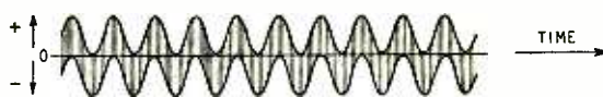
Fig. 3. The two wavy lines represent what is seen of the fixed-frequency ( f_i ) signal; the top one when displaced by a constant positive voltage equal to its peak voltage, and the bottom one when the constant voltage is negative. If an alternating voltage is substituted for the constant one, the combined voltage varies within the shaded area.
