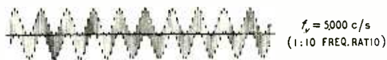
Fig. 10. With f_s = 5,000 , the frequency ratio is the same as in Fig. 4, and the picture the same as in Fig. 4(c) except that everything happens 10 times as often.
