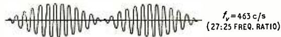
Fig. 9. When f_v is nearly equal to f_f , the time base has to be slowed down to show the beats clearly.
