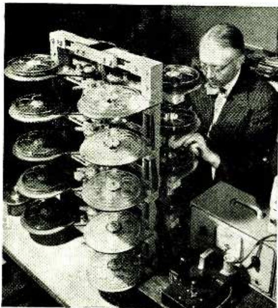
"Multitape" duplicating machine being loaded by Dr. Rawdon Smith, one of the designers.
