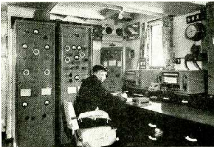
RADIO on the new cable ship "Stanley Angwin" which Cable & Wireless Ltd. put into service last month. She is to be stationed at Singapore. The Marconi equipment shown is (L to R) "Worldspan" and "Oceanspan" transmitters, "Reliance" standby transmitter, shortwave and m-l-wave receivers between which is the remote control for the aerial splitter installation. Radar and echo-sounding gear was supplied by Kelvin & Hughes. D. A. Sydenham is the Radio Officer.
