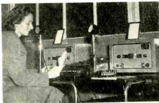
(Right) Pye PTC 704 transmitter-receiver installed by Rees Mace in a tanker. (Below) The control equipment (with microphone and receiver for each fixed station) at the service depot of the Pressed Steel Co.
