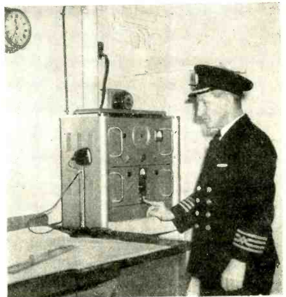
(Right) Pye PTC 704 transmitter-receiver installed by Rees Mace in a tanker. (Below) The control equipment (with microphone and receiver for each fixed station) at the service depot of the Pressed Steel Co.
