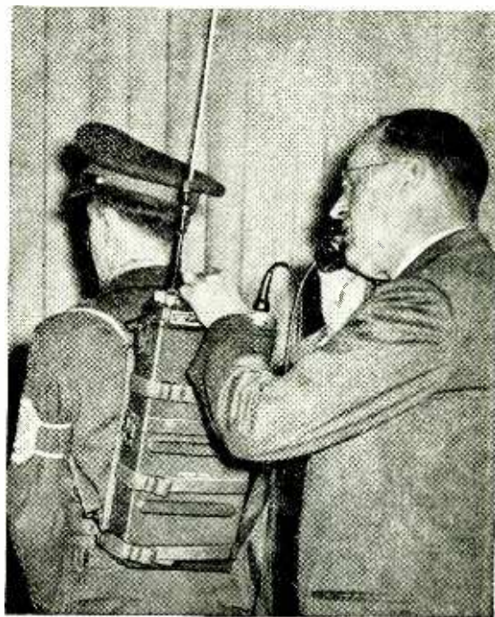
New R.C.A. walkie-talkie designed for the United States Army Signal Corps. This illustration shows the equipment assembled as a pack set.
