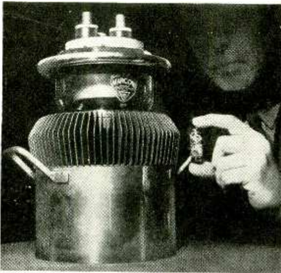
Comparison between the giant BR128 v.h.f. air-cooled transmitting valve and a typical modern receiving valve.
