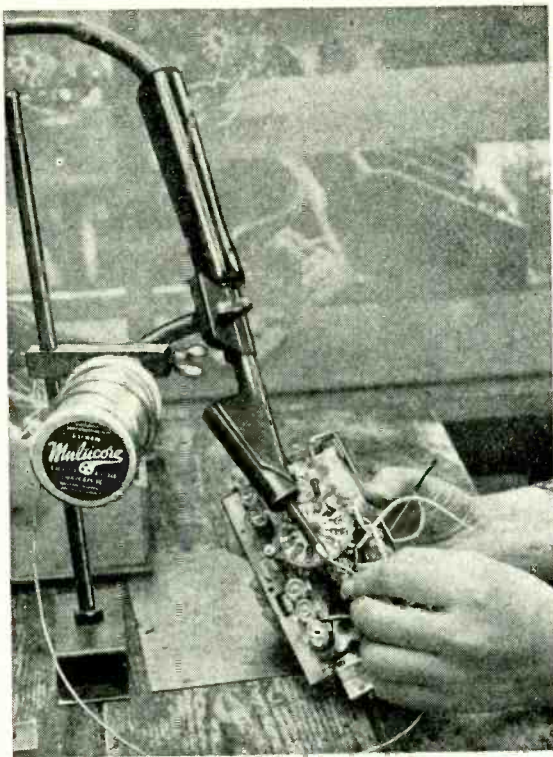
A switch unit for a Pye receiver has 75 soldered joints made entirely with a bench fixed iron. This unusual method of soldering enables a very fine bit to be employed and reduces fatigue on the part of the worker.
