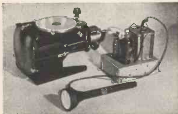
The main components of the projection television system
