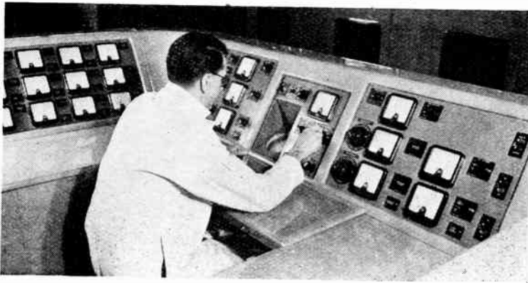
MIDLAND TELEVISION. The vision and sound control desk for the Sutton Coldfield station. The vision transmitter and this control desk are being supplied by E.M.I. and the sound transmitter by Marconi's.
