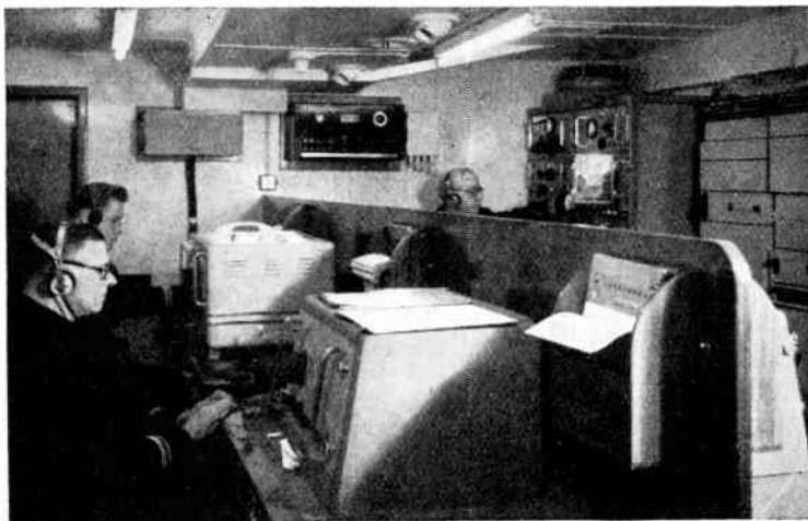
RECEIVING ROOM in the S.S. Caronia showing the W/T receiver and, in the right background, the single sideband receiver.
