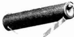
Three type 36EHT35 rectifiers, each only 3" long X 1/8" dia, will, from a peak pulse input of approx. 2,500V obtained from the standard line scanning output transformer, give an output of about 6kV at 100µA, used in the tripler circuit shown on the left.
