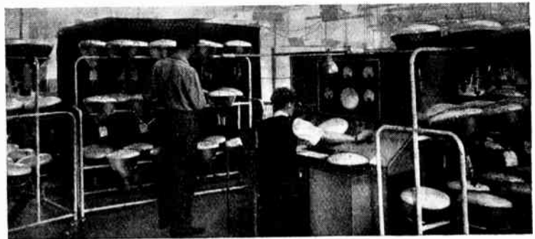
CATHODE-RAY TUBES undergoing a 1,000-hour life test at Ediswan's Ponders End factory forms the subject for this month's cover illustration and twelve-inch tubes are here shown being tested for spot centrality, cathode emission, modulation sensitivity, heater current, and heater-cathode insulation, etc. They are also subjected to an over-voltage test for possible flash-over.
