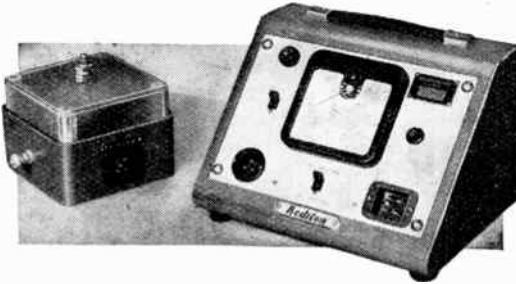
Rediffusion valve kilo-voltmeter Type M36 for measuring R.F. up to 15\text{ kV} and to 30\text{ Mc/s} .
