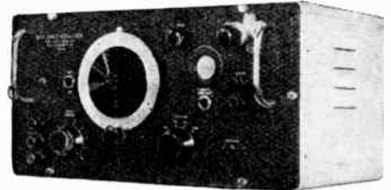
Type 400C A.F. generator covering 0.1 to 1,000\text{ c/s} made by Dawe. This is one of a range extending to 5\text{ Mc/s} .
