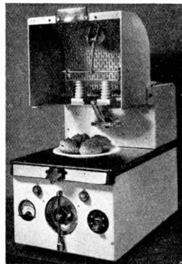
RADIO RE-HEATER. —Intended for re-heating pies, sausage rolls, muffins and other re-heat-cooked snacks (as opposed to cooking from the raw) this equipment, made by Radio Heaters, of Wokingham, works at R.F. on the dielectric heating principle. Power output, 0.5kW; frequency 75Mc/s.
