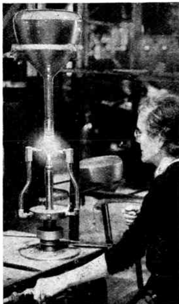
OUR COVER. Two processes in the manufacture of C.R. tubes are given on our front cover an' above; showing, respectively, annealing the neck to the bulb an' sealing-in the electrodes. The photographs were taken at the High Wycombe factory of Electronic Tubes Ltd., a Cossor subsidiary.
