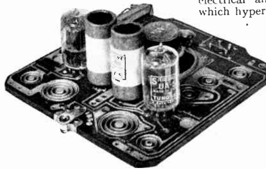
SARGROVE all-stage valves, shown by Tungsram, fitted on a chassis with components "sprayed on" by the E.C.M.E. process.
