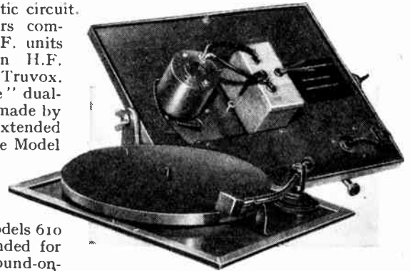
Gramophone turntable driven by two-phase motor (Electrical and Radiological Instruments).
