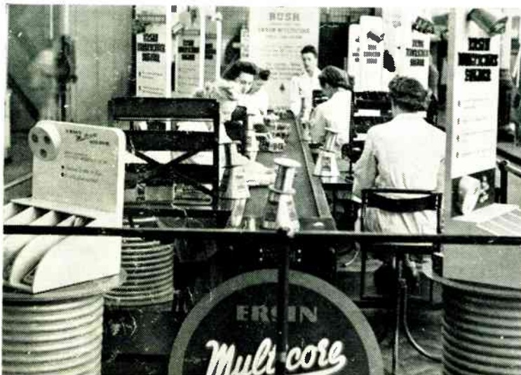
A section of the conveyor on the Ersin Multicore Solder Stand where a complete Bush coil unit was manufactured every five minutes.
