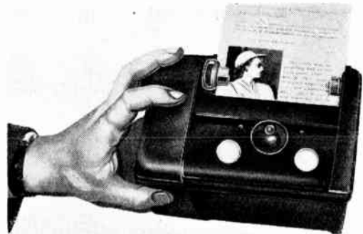
(Courtesy "F.M. and Television") All the actuating mechanism is contained in this facsimile unit for operation from a standard F.M. receiver.
